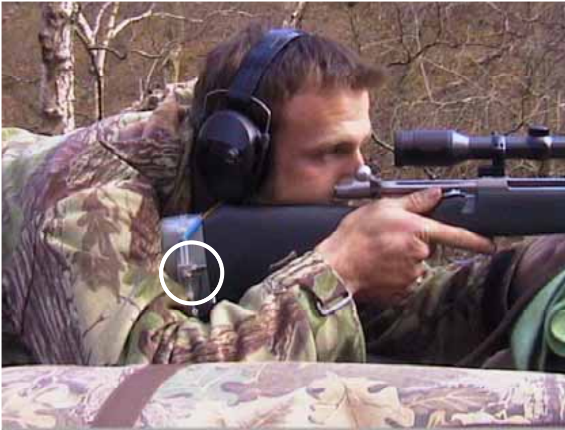
Figure 3 Accelerometers fitted on stock
